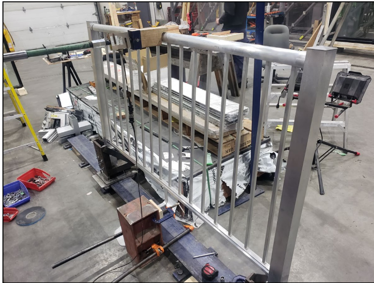
Figure 3. Horizontal –Mid-span of Top Rail Concentrated Load
