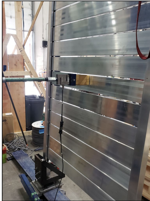
Figure 3. Mid-Span of Privacy Board Concentrated Load
