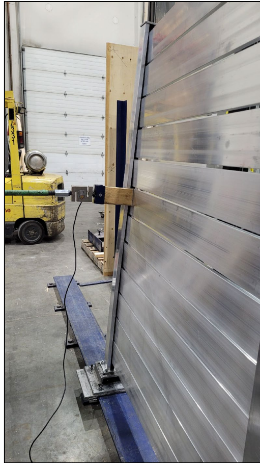
Figure 3. Privacy Wall (Deck Mount) – Horizontal – Adjacent to Post Concentrated Load
