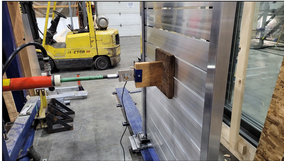
Figure 1. Privacy Wall (Deck Mount) – In-fill Load Test
