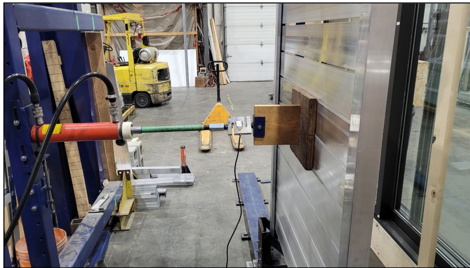
Figure 5. Privacy Wall (Fascia Mount) – In-fill Load Test
