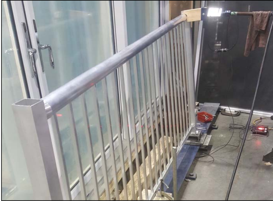
Photo 3. Adjacent to Post Connection Concentrated Load Test
