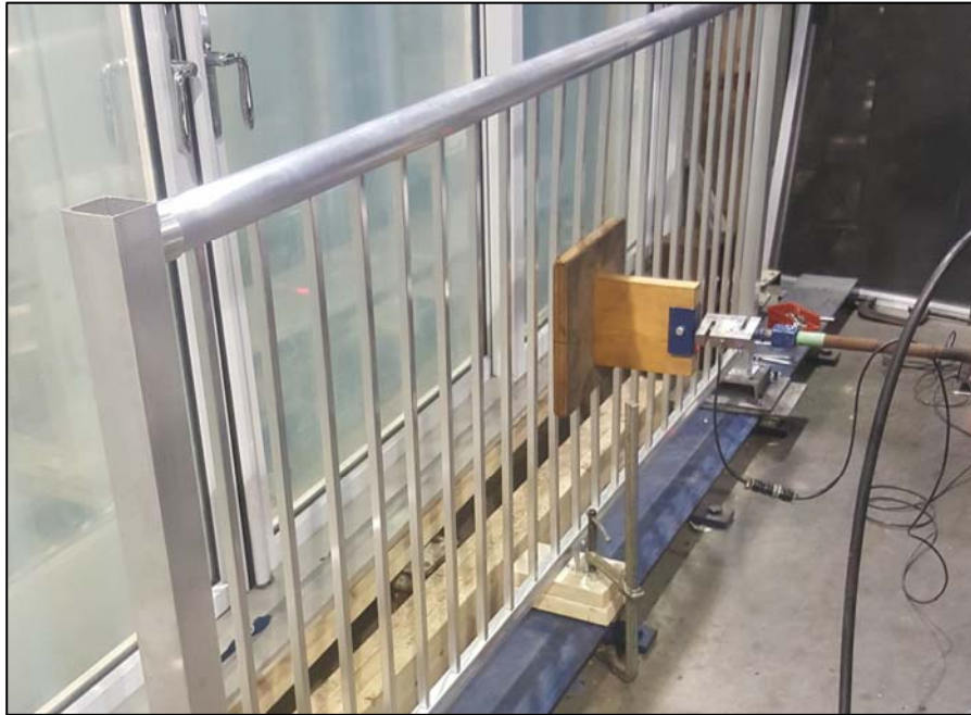
Photo 1. In-fill Load Test
