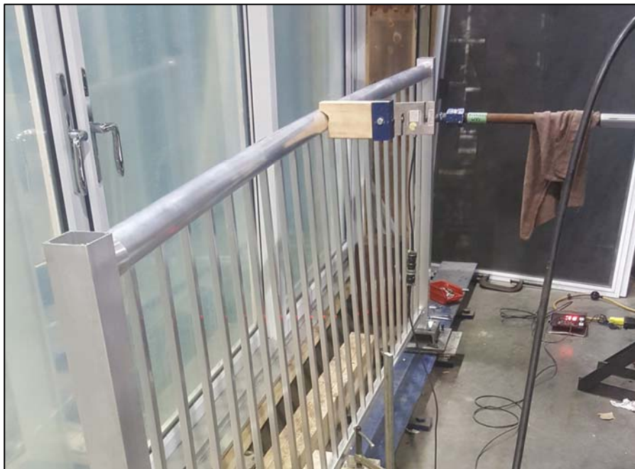
Photo 2. Mid-Span Concentrated Load Test
