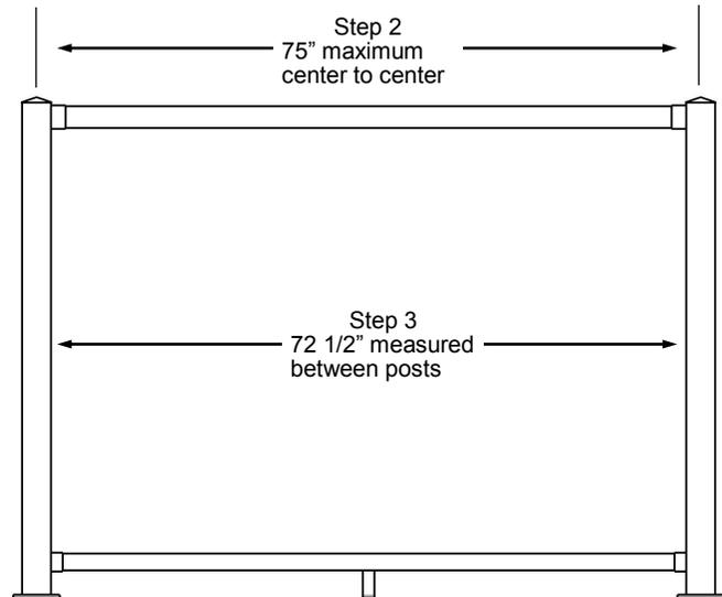
**Step 3:** Measure distance between inside of posts and deduct 3" from total measurement. ie: post to post measurement = 72 1/2".
