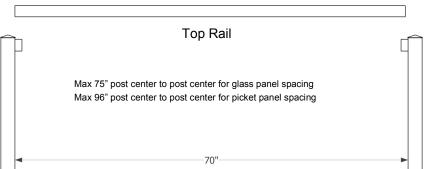
measure the distance between the posts (for accuracy, take measurement between both posts at the bottom), subtract 5/8" from total measurement, and cut top rail.
