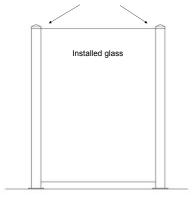
When Scenic Railing is being used as a guardrail, do not exceed the 48" center to center spacing as this is outside our engineering spec and is at the end users own risk and could result in a failed inspection. It is the sole responsibility of the home owner/contractor to comply with local building codes.
