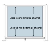
Lubricate top and bottom rail glass insert with soapy water. Install glass by holding the 37 5/16" sides of the glass (for 42"rail) and insert into the top rail channel as far as possible. Swing the bottom of the glass over the bottom rail until its centered over the bottom channel. Pull down on the glass until it slides into the bottom channel and is sitting on the two rubber blocks inserted previously. Centre the glass between the two posts by sliding it the the left or right.
