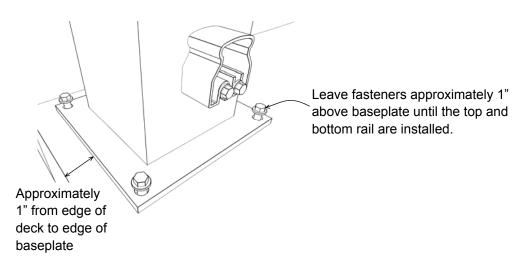
When Century Railing is being used as a guardrail, do not exceed the maximum span stated for the various types of railing as this is outside our engineering spec and is at end users own risk and could result in a failed inspection. It is the sole responsibility of the home owner/contractor to comply with local building codes.
