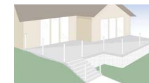
STEP 1 Layout post locations, leave lags 1" up from baseplate
