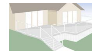
STEP 2 Cut and attach top and bottom rails, secure posts
