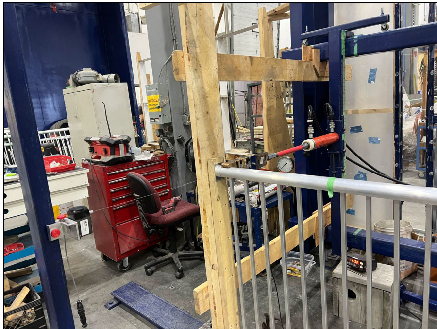
Figure 8 – Wall Bracket Mount – Adjacent to Post Concentrated Load Test
