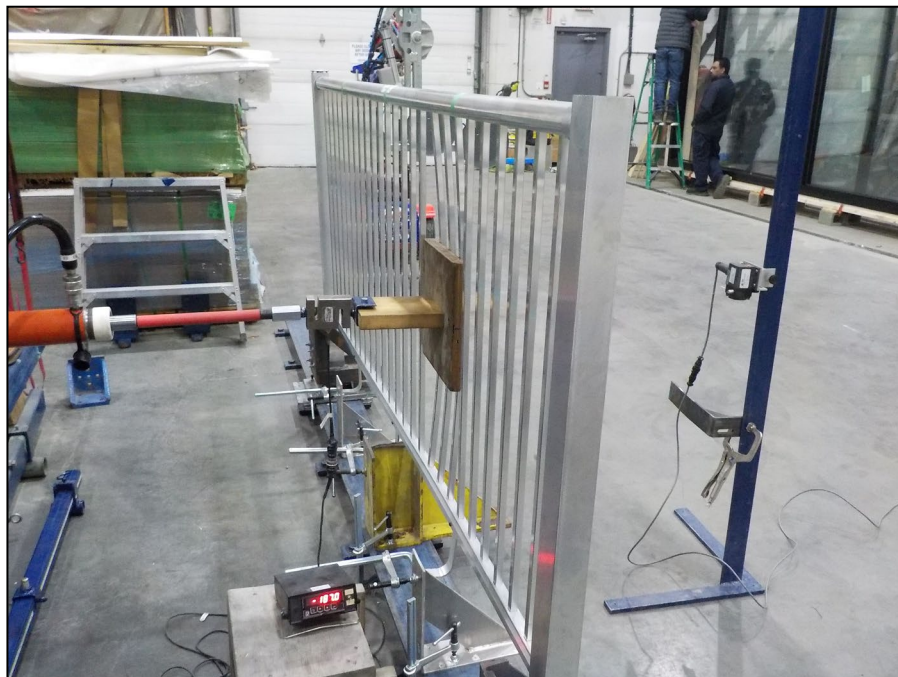
Figure 4 – Fascia Mount – In-fill Load Test
