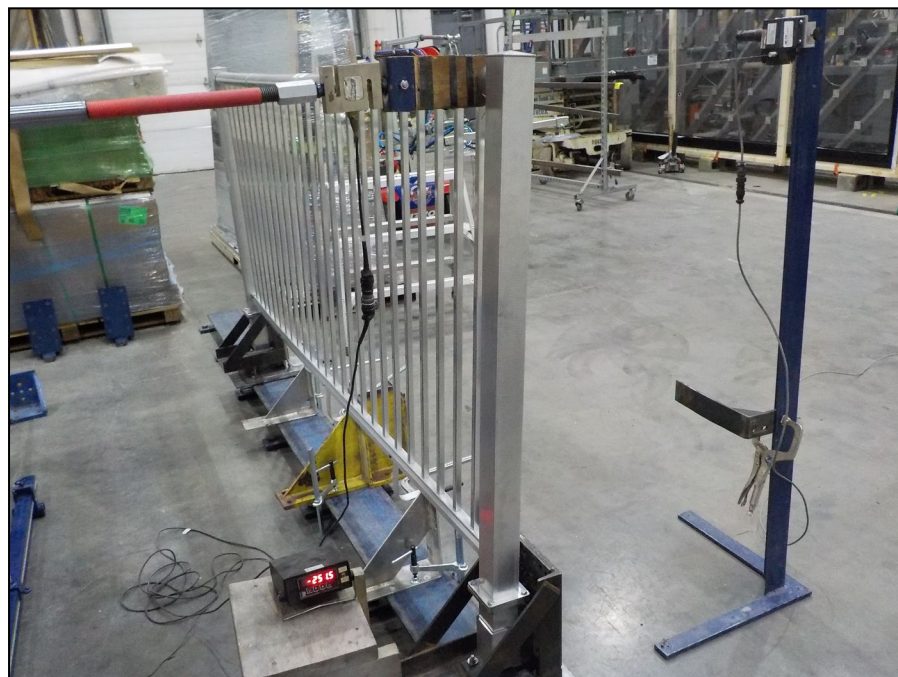
Figure 6 – Fascia Mount – Adjacent to Post Connection Concentrated Load Test
